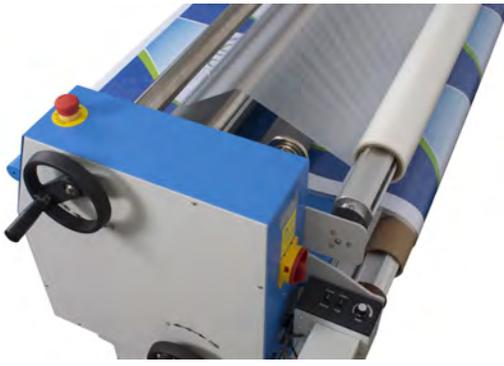
Motorized rear rewind for roll-to-roll applications included.
