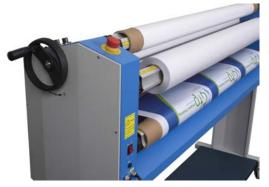
Integrated Rear Rewind makes Roll-to-Roll applications easy.
